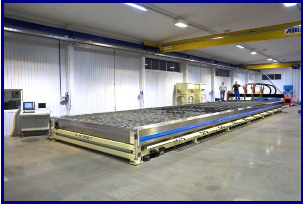
The Water Jet Sweden NC 40180 T Profiler with three cutting heads and a cutting workbed area of 18 metres in length x 4 metres width.
