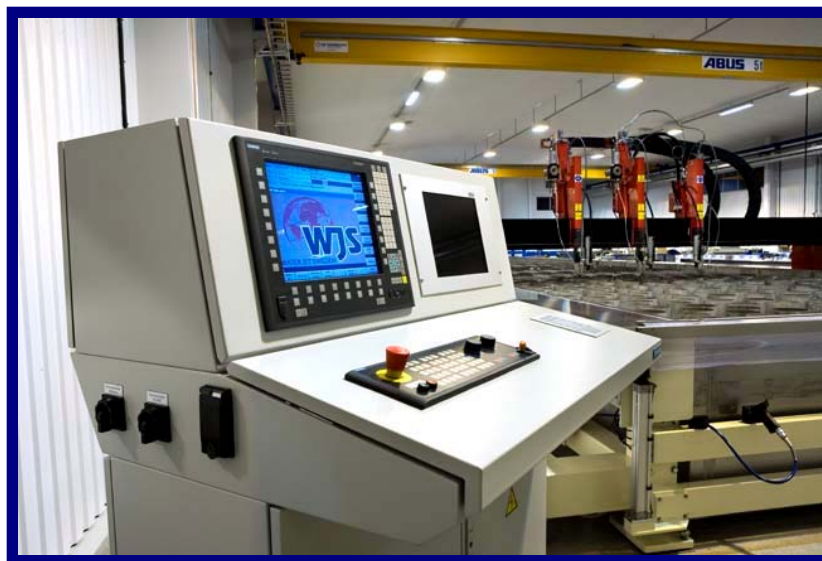
The newly-developed and specially-adapted Siemens 840D CNC console system
