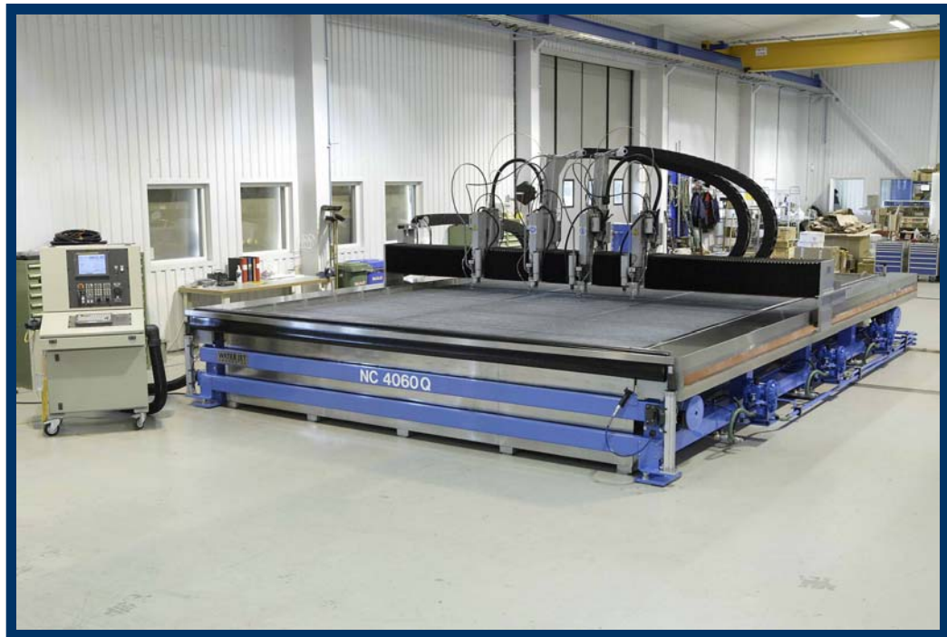
Picture shows one of the new WJS four-headed linear drive machines, model NC 4060Q, especially suitable for multi-head, common line cutting
