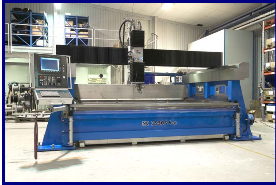
Picture shows one of the new super-accurate 5-axis Water Jet Sweden NC 3520 S cutting machines.
